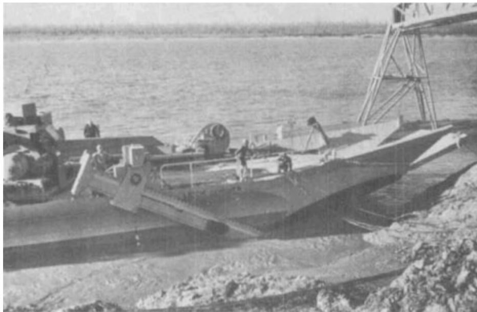
An amphibious ship; the rack and pinion leg walks it ashore.
