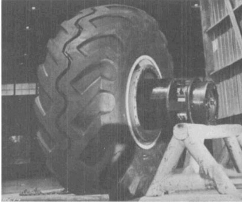
The electric, self-propelled, rubber-tired wheel.
